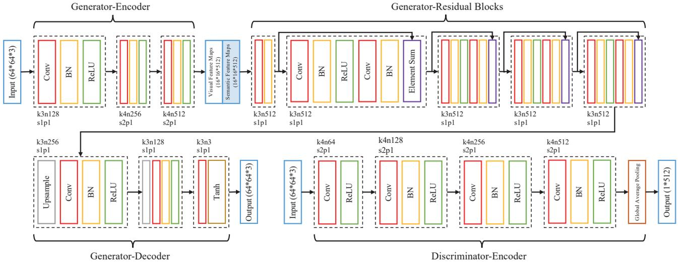
Figure 3: Details of the generator and the discriminator in AMGAN, where  $k$  represents the kernel size,  $n$  represents the number of channels,  $s$  denotes the stride, and  $p$  refers to the padding.
